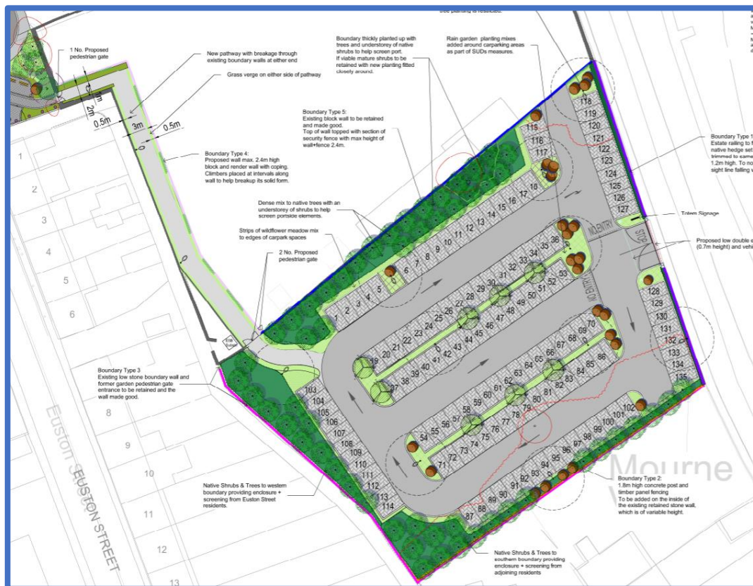
Figure 2.20 Surface Car Park Proposals including pedestrian path to Euston Street (Extract from Drg. No. 103-A Rev N prepared by CSR)
