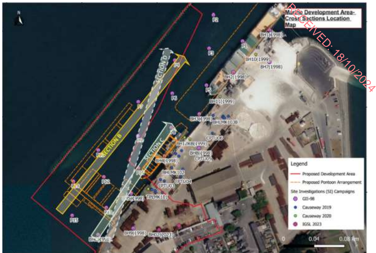
Figure 9.15 Nearshore Development Area – Cross Section and SI Location
